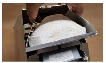
4. Insert the new Element by squeezing the legs on the bracket to clear the tabs on the housing. Ensure the ears on the element bracket are placed on top of the housing tabs.
