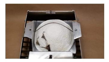
5. Attach the power supply leads to the element leads using the original screws and nuts.
