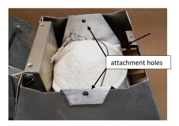
S3 Install the new element so that the bracket tabs hang over the housing attachment holes.
